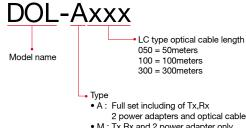
M : Tx.Rx and 2 power adapter only (excluding of optical cable)
